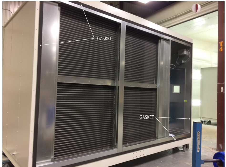
FIGURE 2: GASKET APPLIED TO THE PERIMETER OF THE OPENING ▼
