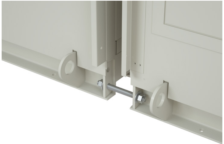
FIGURE 4: THREADED ROD, WASHERS AND NUTS FOR PULLING SECTIONS TOGETHER ▼
